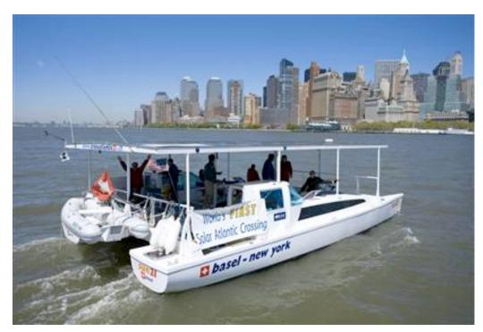
Powered by solar panels atop its awning, the "sun21" approaches Manhattan on Tuesday, ending the crossing that made it the first solar-powered boat to navigate the Atlantic.
